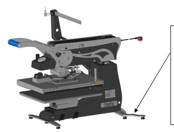
MONTER LA RALLONGE PIED AVANT DE RETIRER LA VIS D'EMBALLAGE MOUNT EXTENSION FOOT BEFORE REMOVING THE TRANSPORT SCREW
